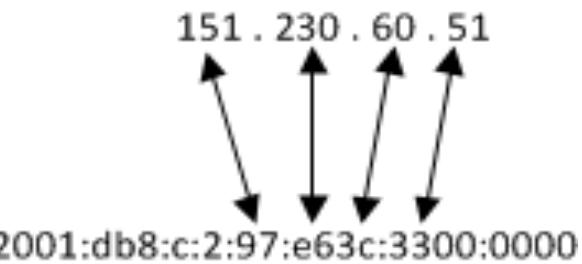
RFC6052 IPv4-embedded IPv6 addresses used for external host destination address.
